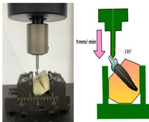
FIGURE 3: Set up of the set-up of the mounted post and core for fracture resistance test in Universal Testing Machine (Shimadzu, Japan) and schematic drawing for fracture resistance test
