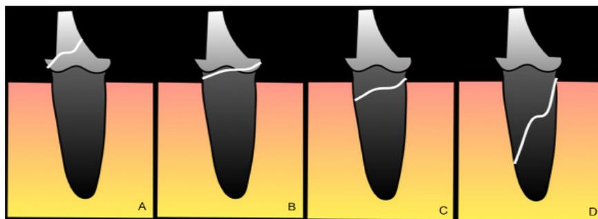
FIGURE 4: Schematic diagram of classification of failure mode. Favourable fracture: A. Core fracture; B. Fracture above the simulated bone level. Unfavourable fracture; C. Fracture below simulated bone level; D. Longitudinal fracture along the root
