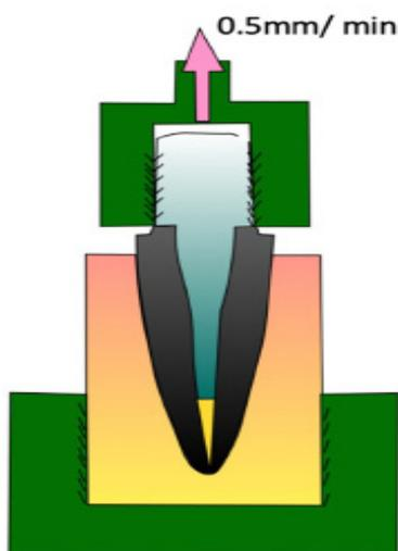
FIGURE 5: Schematic drawing of mounted post and core set-up for retention test
