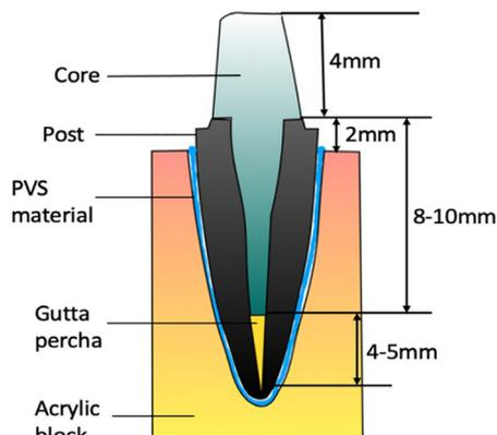
FIGURE 1: Schematic diagram of the specimen's preparation in CG, NC1 and VE1 group. The specimen in NC2 and VE2 groups were mounted in acrylic resin blocks without PVS impression materials
